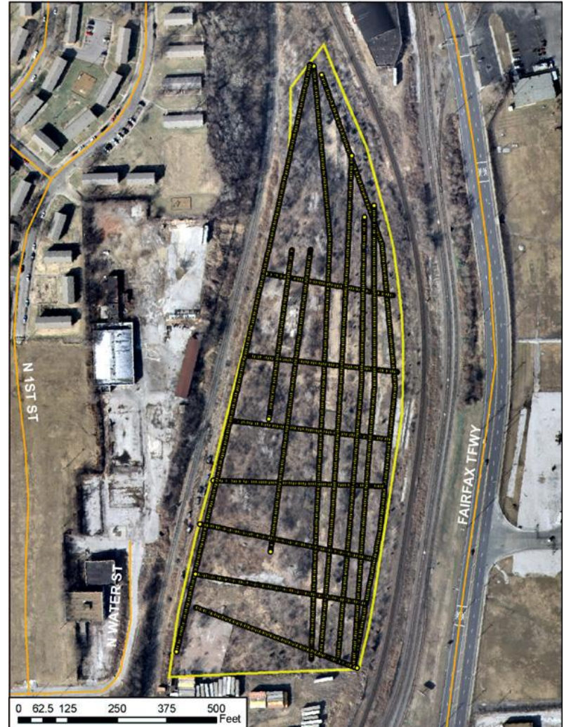
ERI: Electrical Resistivity Imaging
