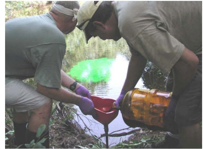
Fluorescent Tracer Testing
