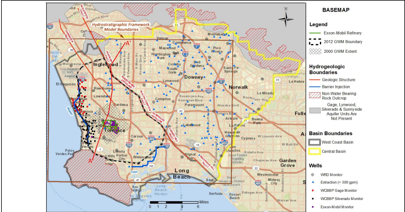
Groundwater model domains and boundaries of the hydrostratigraphic framework model constructed to provide the conceptual basis for the revised groundwater model, boundaries of the Central and West Coast Basins, lines representing the West Coast Basin Barrier Project (WCBBP) and Dominguez Gap Barrier Project (DGBP) injection wells, and the monitoring and injection wells from which data was used for model construction and calibration.
